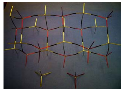
Fig. 1. Mockup of the CL structure. Individual CL nodes formed by 4 prisms are separated by gaps (black line)
