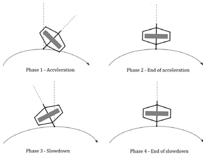
Fig. 11. Phases of gyroscope orientation relative to trajectory
