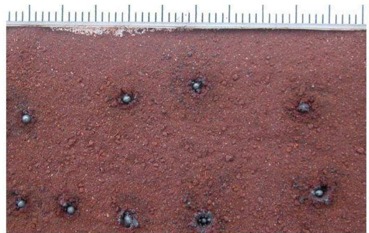
Fig 3. Set of spherules formed by plasma discharge contacting hematite.
