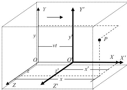
FIG. 2. Coordinate transformation in a moving medium.
