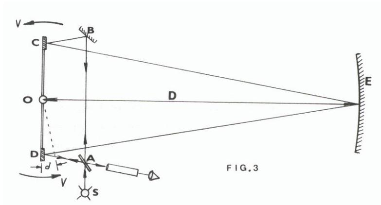
The light beam from a source S was split by a semi-transparent mirror A. The one beam continued through mirror A to mirror B, and was reflected to mirrors C, E and back via mirror D to A. The other beam was reflected from mirror A to mirror D and then in opposite direction via D E C B to mirror A, at which point it was superimposed on the first beam to obtain a fringe pattern when the mirrors were properly adjusted.
