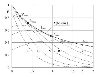
Figure A1.3-2. Transmission curves obtained by numerical integration of (58) for filters UBVRIZJ for radiation in the redshift range z = 0...2 from a blackbody with  $\lambda_T = 350$  nm ( $\lambda_W = 440$  nm, T = 8300 °K). Each curve touches the bolometric curve of equation (57) at the redshift matching maximum of the radiation flux to the nominal wavelength  $\lambda_W$  of the filter (small circles in the figure).
