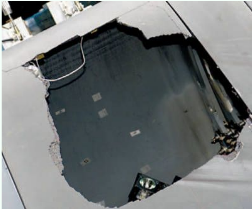
The large impact hole in Panel 8 from the final test.
