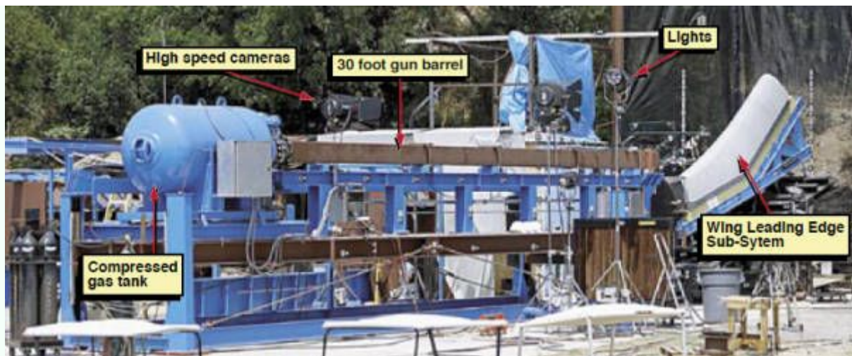
Nitrogen-powered gun at the Southwest Research Institute used for the test series.
