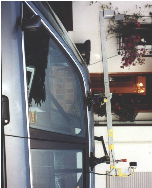
Fig. 9. Photo showing the Measuring Gauge Mounted on the Car's Top in 2000
