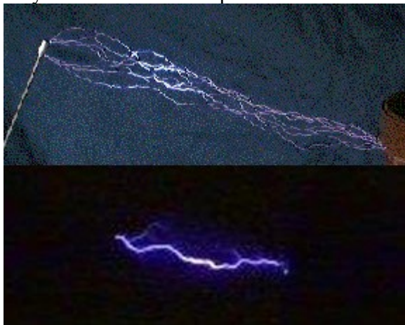
Figure 1. Spark discharges from a Tesla coil showing greater intensity in the center.
