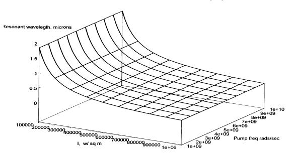
Fig 3. Resonant wavelength (microns) for a range of pump frequency from  $10^9$  to  $10^{10}$ s/sec and a range of beam intensity from  $10^5$ to 10<sup>6</sup> Watts/m<sup>2</sup>.
