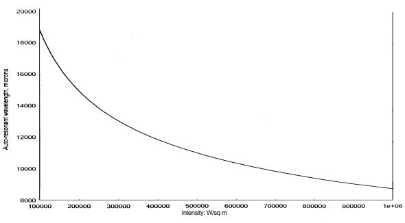
Fig 4. Auto-resonant wavelength (microns) as a function of beam intensity, Watts/m<sup>2</sup>.
