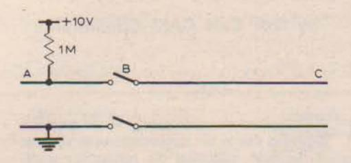
A five-volt pulse two metres wide was found to travel off to the right at the speed of light for the dielectric on closure of the switches, leaving the section AB completely discharged. (The practical device lacked the second, lower switch at B, which is added in the diagram to simplify the argument).
