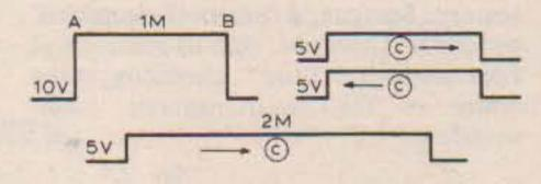
This paradox, that when the switches are closed, energy current promptly rushes away from the path suddenly made available, is understandable if one postulates that a steady charged capacitor is not steady at all; it contains energy current, half of it travelling to the right at the speed of light, and the other half travelling to the left at the speed of light.
