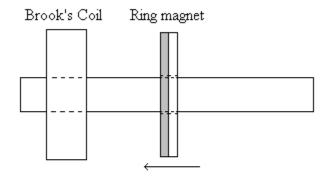
With AC current in the Brook's coil the ring magnet "inches toward the coil
