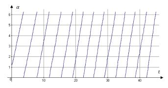
**Fig. 6.** Dependency of the angle a between spin axis of the gyroscope and the polar axis
