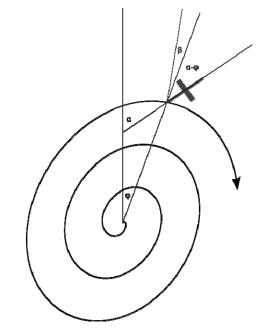
Angle  $\beta$  between radius-vector  $\vec{r}$  and normal line to a spiral is calculated using Eq. (1)
