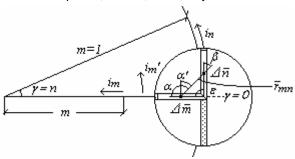
Figure 4 – The m=1,  $n=0^{\circ}$  Singularity With  $\Delta m = \Delta n$ ,  $r_{mn}^2 = 0.5 \Delta m^2$ ,  $\varepsilon = 90^{\circ}$ ,  $\alpha = 135^{\circ}$  and  $\beta = 45^{\circ}$  for  $i_m$  and  $i_n$  in M-mode; and  $\varepsilon' = 0^{\circ}$  and  $\alpha' = \beta = 45^{\circ}$  for  $i_m'$  and  $i_n$  in G-mode (see
