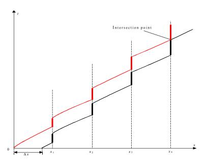
Fig. 1. An intersection of the right and left light pulses at the point  $x_n$  for n = 4.
