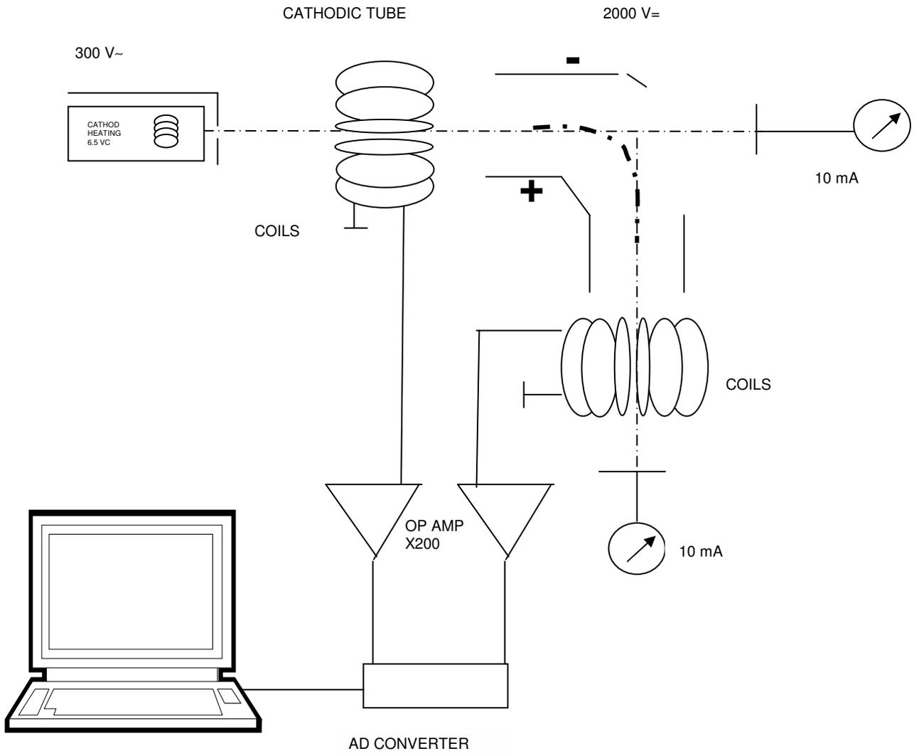
Example of a modified Narva PR2 Tube used by the author to measure the magnetic field of an electron beam magnetic field. The tube of the new experiment proposed by this paper shall be bent by  $90^\circ$  in the middle.
