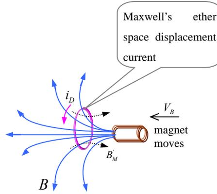
Figure 6, time variable magnetic field generates time variable electric field, which is generating time variable displacement current  $i_D$ ,  $i_D$  generates opposite direction magnetic field  $B'_M$
