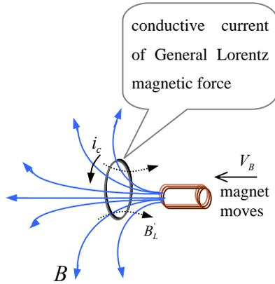
Figure 5, bent moving magnetic lines cut metal electrons, which generates inductive current  $i_c$  under General Lorentz magnetic force, and  $i_c$  generates the opposite direction magnetic field  $B'_L$
