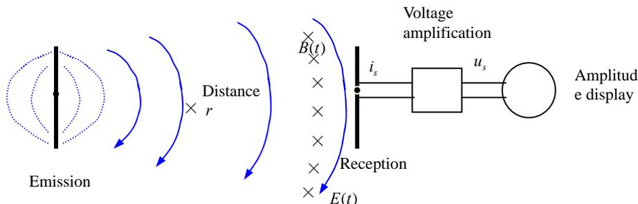
Figure 5 Figure of the emission and reception of the electric wave----field vector radiation
