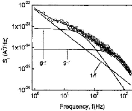
Fig. 1. Example of  $1/f$  noise in the picoampere current range from a diode rectifier, along with contributed noise (g-r lines) from two quantum dot devices (Tsormpatzoglou, 2005).
