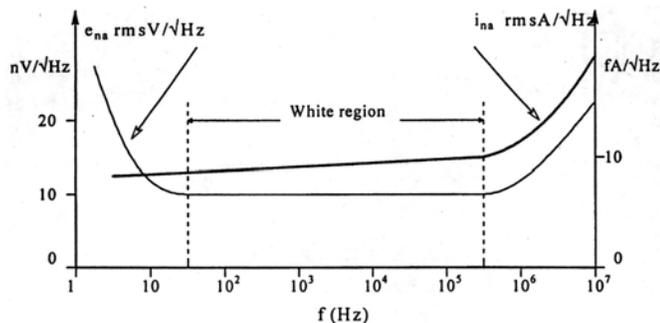
Fig. 8. Plots of typical input noise root power spectrums for an FET input amplifier (Northrop, 1997).
