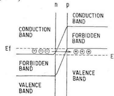
**Fig. 6.** Tunneling current in a reverse-bias, backward tunnel diode used as a rectifying device at zero bias (Morizuka, K., "Rectifying device for achieving high power efficiency," U.S. Patent 5,930,122, July 27, 1999, Fig. 5)
