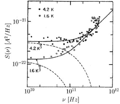
Fig. 2. Measured spectral density of current noise in the shunt resistor of Josephson junction at 4.2K (solid circles) and 1.6K (open circles) up to 500 GHz. Solid lines are the prediction of Equation 2 while the dashed lines represent the theoretical prediction in the absence of the zero-point energy term and fall far below the data at the higher frequencies (Koch, 1982).
