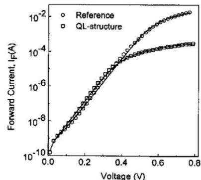
Fig. 9. Experimental forward current-voltage characteristic of a typical Au/n-GaAs Schottky diode for a reference GaAs sample
