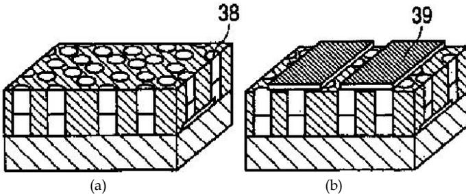
**Fig. 4.** Updated version of a Brown's p-n junction (a) diode array (38) and (b) with parallel conductors (39) added (Kuriyama, A., Miyata, H., Otto, A., Ogawa, M., Okura, H., Fukutani, K., and Den, T., "Method for Manufacturing a Semiconductor Device", U.S. Patent 7,183,127, Feb. 27, 2007, Fig. 4D and 4E).
