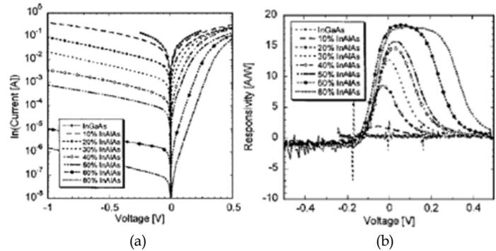
**Fig. 5.** Example of a modified Schottky diode (semimetal-semiconductor) InGaAs rectifier for sensitive room-temperature microwave detection that operates well at zero bias voltage, where (a) shows increasing current levels in amperes with lower InAlAs percentage and (b) shows increased responsivity in A/W at zero bias voltage and higher InAlAs levels (Young, 2005).
