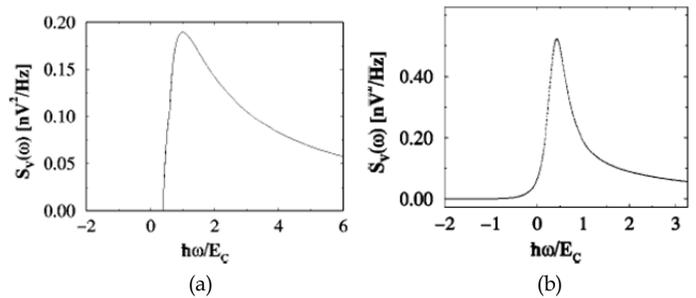
Fig. 3. Spectral density of voltage noise in a single-electron transistor (a) in the off-state as compared to the (b) normal run mode at 1.5 nA and  $E_c = 2.5$  K (Kach, 2003)
