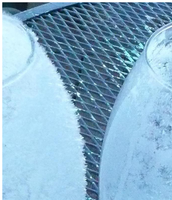
Fig. 1. Formation of frost within the mirror at left vs. control, right
